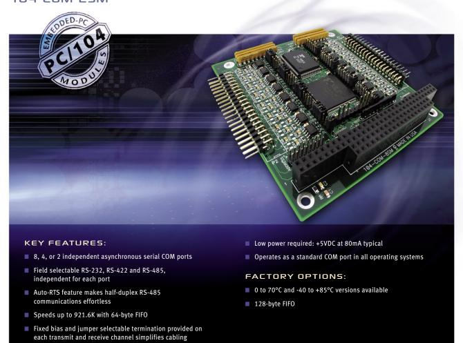
The 104-COM-8SM Series are eight, four, or two-port, asynchronous, serial communication boards that support field selectable RS-232/422/485 communication. Ports are accessed via two 40-pin IDC type right angle header connectors. The boards include a convenient Auto-RTS feature, which makes half-duplex RS-485 communications effortless.
